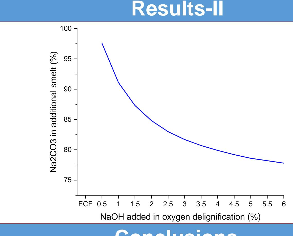
The extent of  $CO_2$  capture in recovery boilers can be increased via sodium spiking, and the opportunity exists to lower costs of CO<sub>2</sub> sequestration via increased capacity in the lime kiln.
