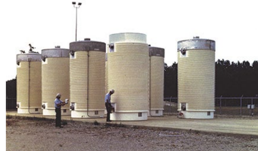
Dry storage casks
