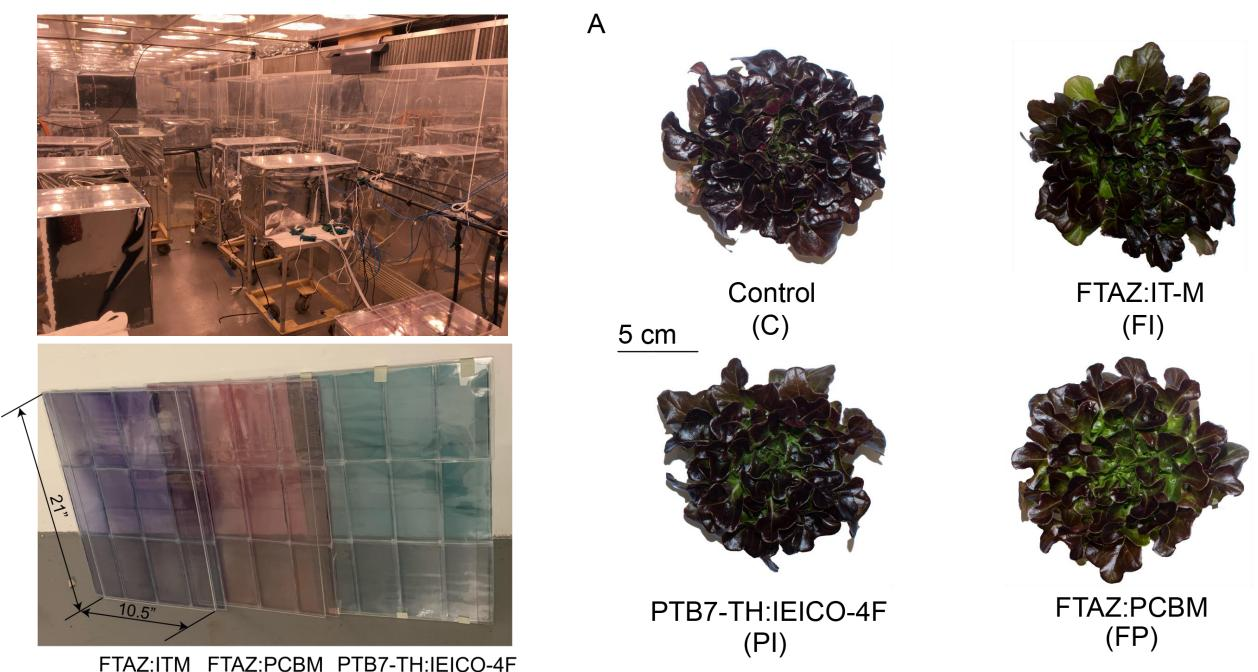
A solar powered greenhouse would utilize sunlight for both plant growth and energy production. Our purpose is to develop a self-sustaining greenhouse system that utilizes organic solar cells (OSC) to selectively filter certain wavelengths for energy production, while allowing wavelengths critical for plants to pass through.
