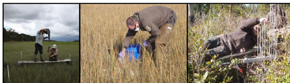
Photos: Installing a rod surface elevation table benchmark at Blackbeard Island NWR (credit: Dave O'Loughlin/Atkins); establishing accretion plots within tidal smooth cordgrass zone on Wolf Island NWR (credit: Nicole Rankin/USFWS); measuring surface elevation from rod surface elevation table benchmark installed in pocosin wetlands at Pocosin Lakes NWR (credit: Nicole Rankin/USFWS).
